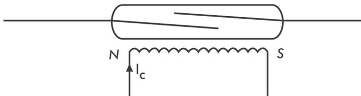
**Fig.4: A dry reed switch biased by a permanent magnet and operated by a coil**
