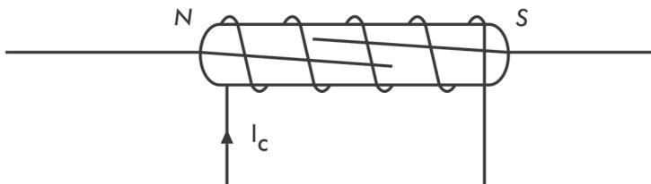
**Fig. 3: A dry reed switch mounted outside a coil**
