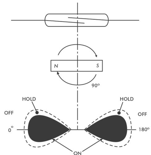
**Fig. 7: Rotational movement with a bar shaped permanent magnet**
